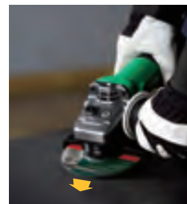
Motor stops due to overloading.
