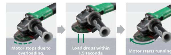
\*5. The motor may not automatically restart when the kick-back protection is activated or for other safety reasons. In that case, the tool needs to be turned off and on manually.
